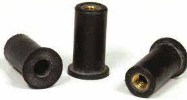
The RivetKing JF Series Rubber Nut are used as a removable rivetnut. Installation is performed with the bolt or screw itself. To remove the rivet nut, just remove the bolt or screw. Rubnuts can also be used as vibration isolators to prevent the rattle and pullout. Typical applications are for the installation of mirrors or other hardware in utility trucks, compressors, and engines.
